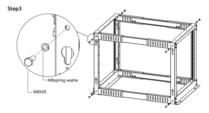
Assemble the side beams and uprights with hexagonal M8\*20 screws and M8 spring washers. Repeat the above actions for a total of 8 places.
