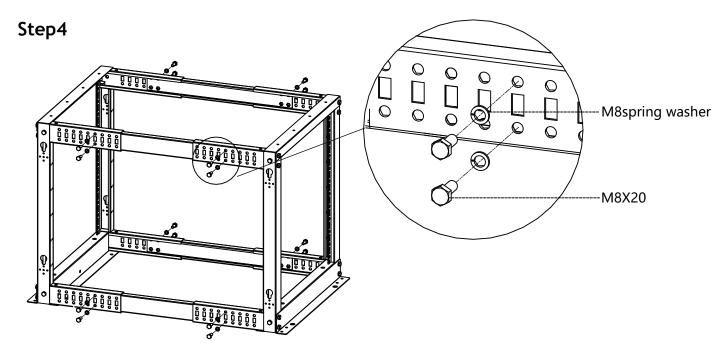
Select the desired depth according to the table on the right, then assemble the side beams with the side center beams and repeat the above for a total of 8 places.
