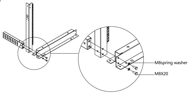
Assemble the side beams, columns and base plate with hexagonal M8\*20 screws and M8 spring washer. Repeat the above for a total of 4 places.
