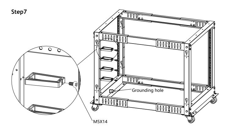
After aligning the cable management ring positioning holes with the holes on the uprights, screw in the front with the M5X14 screws, taking care not to over-tighten them.
