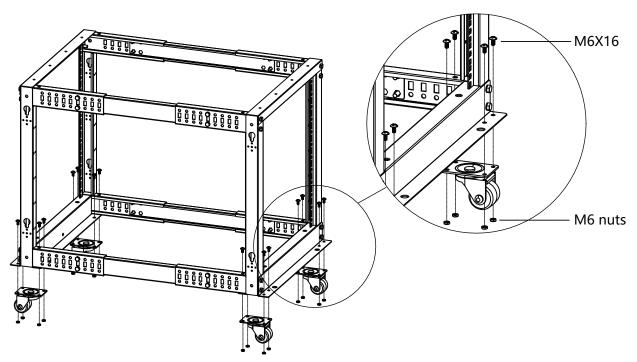
Assemble the caster with Phillips M6\*16 screws and M6 nuts. Repeat the above for a total of 4 places.
