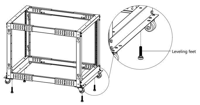
Just screw the leveling feet until they are flush with the casters. Repeat the above for a total of 4 places.
